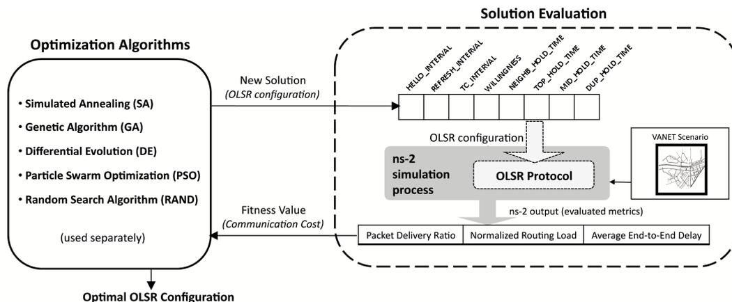
Figure 1: Optimization framework for the automatic OLSR configuration in VANETs. The algorithms invoke the *ns-2* simulator for each solution evaluation.
